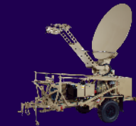
Satellite Transportable Terminal (STT)
